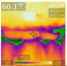
Infrared picture of bathroom ceiling. Green areas indicate surface temperatures below the dew point. Coldest surface temperature measured at 35.1F.
