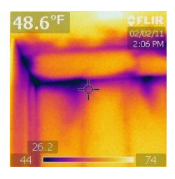
Simulated 30% RH and IAT at 72F in software. No surface temperatures indicate dew point.
