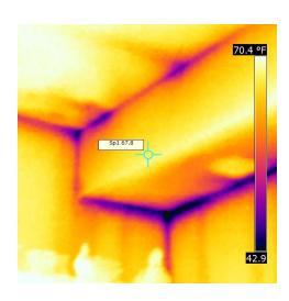
Simulated 35% RH and IAT at 72F in software. NW corner and small spot on N wall indicate dew point reached.
