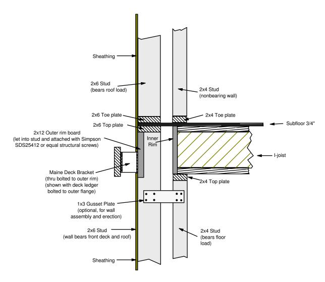
Detail of East Wall Between Floors (View Perpendicular to Joists)
