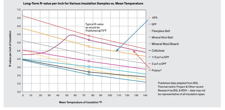
Figure 2. Thermal Resistance versus Insulation Mean Temperature
