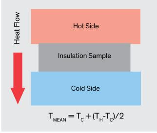
Figure 1. Thermal Resistance and Mean Temperature
