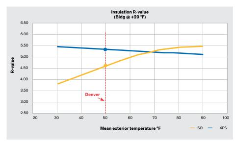
Figure 5. Effective R of Roofing ISO and STYROFOAM<sup>™</sup> for Building Maintained at +20°F
