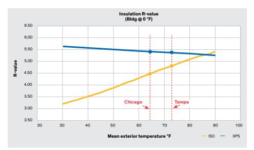
Figure 4. Effective R of Roofing ISO and STYROFOAM<sup>™</sup> for Building Maintained at 0°F
