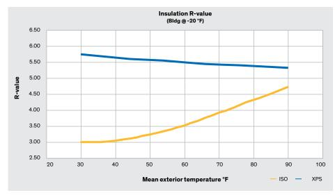
Figure 3. Effective R of Roofing ISO and STYROFOAM  $^{\scriptscriptstyle \rm M}$  for Building Maintained at -20°F
