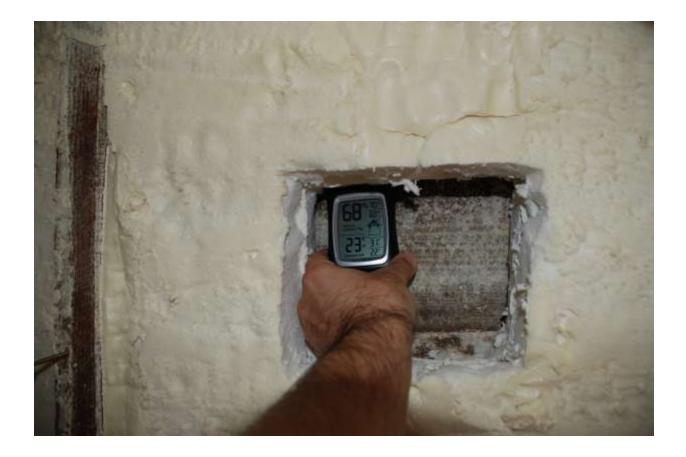
You can clearly see same temperature but much higher RH. The absolute moisture difference behind foam vs. interior side vs. outdoors appears to be fluctuating. BTW, the hole was covered with the foam pieces I cut out and the thermometer was stuck between planks and foam.
