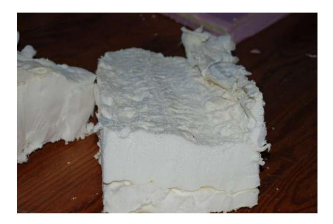
Above you see again two layers, and it's a foam piece called "Prince" with a "perm" ③. The top is the exterior side, which should have been <u>flat</u> but instead, at the right it sticks out almost 2". This clearly shows the foam wasn't applied correctly.
