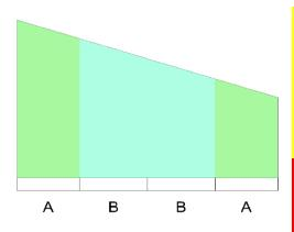
The illustration on the left shows the required screw spacings based on the loading. For the spacing the weight of the buildup as well as wind preassures/suction has been considered. The inindividual areas like (A) and (B) in the illustration would consider different wind pressures on the corner compared to the center of the wall. IN this case (and the entire project) the spacings are identical for all areas of the wall.
