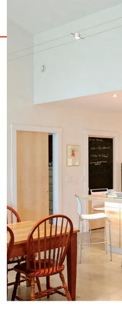
Passive solar. The south-facing, triple-glazed Intus windows are Passive House certified. The low-maintenance concrete floors store heat from the sun.
