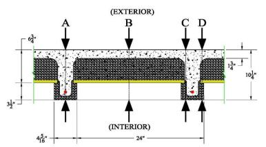
All EPS insulation used in this example is assumed to be 1.5 lb. density rated R-4 per inch.
