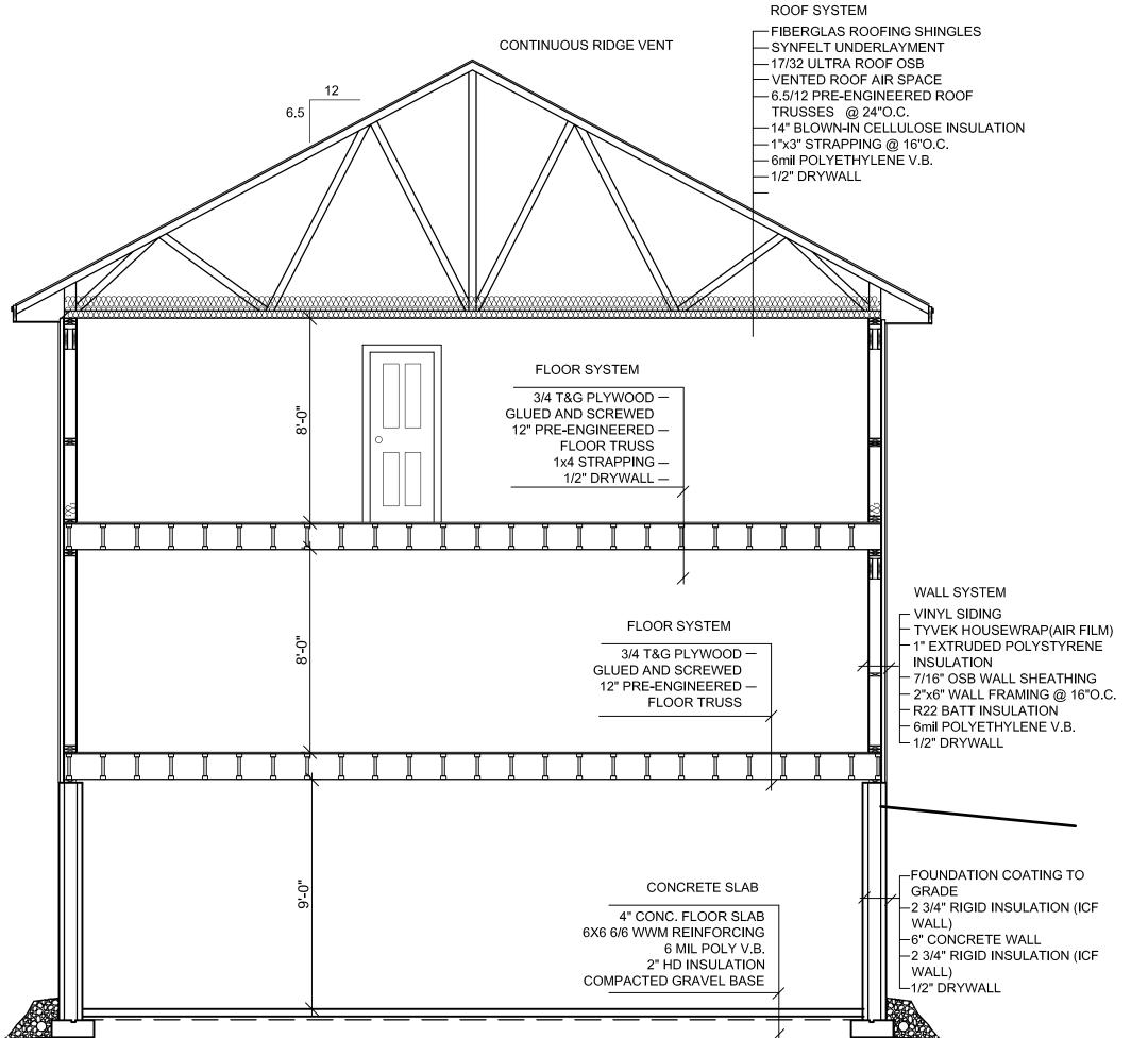
—1/2" DRYWALL FLOOR SYSTEM - 3/4 T&G PLYWOOD GLUED AND SCREWED - 12" PRE-ENGINEERED FLOOR TRUSS - 1x4 STRAPPING – 1/2" DRYWALL FLOOR SYSTEM 3/4 T&G P↓YWOOD — GLUED AND SCREWED 12" PRE-ENGINEERED -FLOOR TRUSS CONCRETE SLAB 4" CONC. FLOOR SLAB 6X6 6/6 WWM REINFORCING 6 MIL POLY V.B. 2" HD INSULATION COMPACTED GRAVEL BASE
