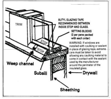
under the glass fills with water so as to immerse the glass seal constantly, the 10 year warranty will be void, as this condition will make premature seal failure very likely. If you use two setting blocks, there should be three weep channels (one for each space under the glass) and if three setting blocks are used, there should be four weep channels.
