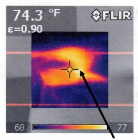
Missing insulation was noted in the attic which will also cause warm interior air to mix with cold attic air.
