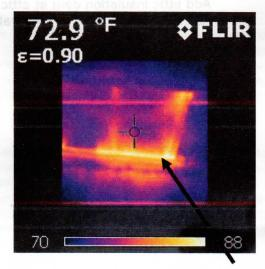
Attic air leakage through attic hatch. Trim should be caulked and hatch should be insulated and weatherstripped as required.
