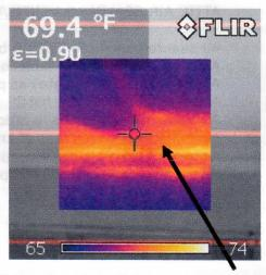
Extensive air leakage was noted at the exterior top plates which need to be air sealed.
