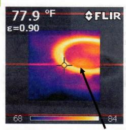
Attic air leakage through can lights. Housing in attic should be covered and air sealed.
