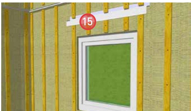
15. Install ROXUL® COMFORTBOARD™ 80 and secure with strapping. Provide bugscreens at the top and bottom of the strapping.
