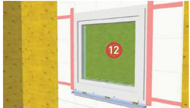
12. Install sheathing tape along the jambs of the window frame and extend to the face of the wall.
