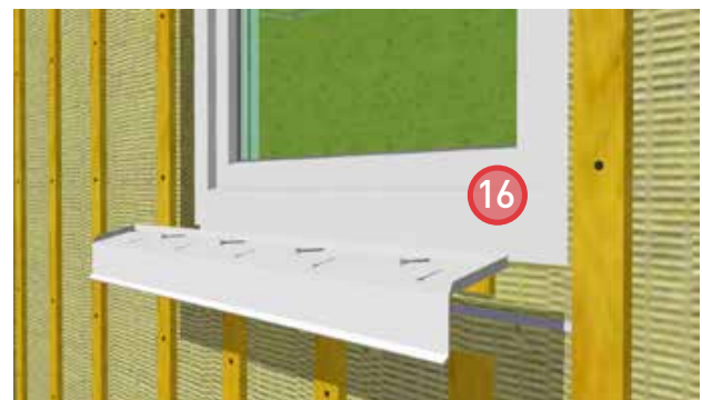
16. Install prefinished metal sill flashing. Attach the sill flashing to the nailing flange under the window sill.
