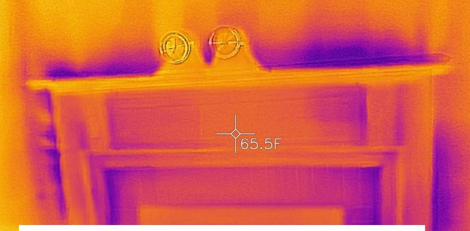
This photo shows my mantel air leakage at steady state with no blower door. Same type of leakage at floor to wall intersection. Looking for exterior air sealing detail and advice to solve this.
