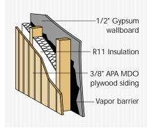
curing conditions. And MDO plywood siding contributes to the thermal resistance of walls.
