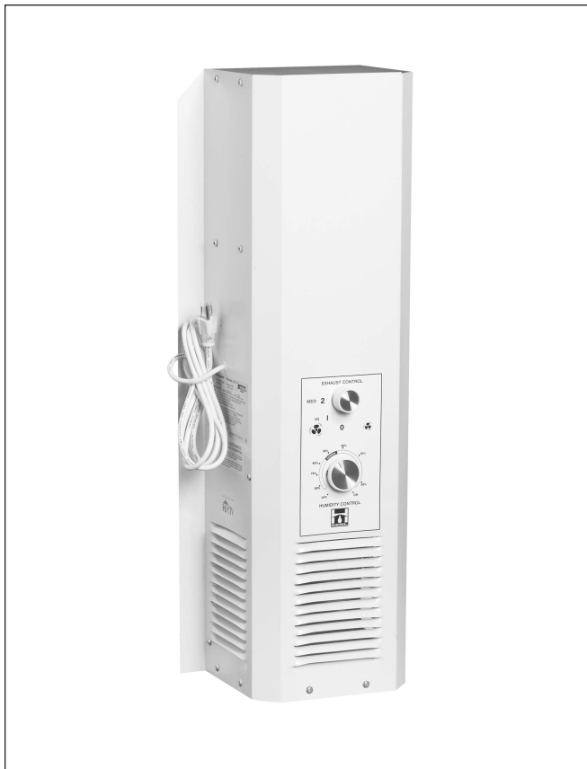
Figure 5. The Humidex crawlspace exhaust fan is housed in a cabinet that measures 7 inches deep by 11 inches wide by 30 inches tall. In a low (e.g., 24-inch-high) crawlspace, the manufacturer recommends installing the unit at an angle.
