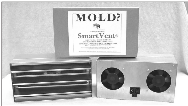
Figure 10 — Each Smartvent unit, which is sized to replace a standard 8x8x15 inch concrete block, includes two fans with a combined rating of 295 cfm.
