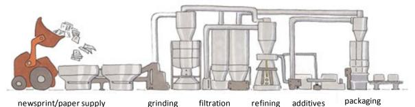
Figure 2: Cellulose insulation manufacturing (NrGaïa website, 2013)
