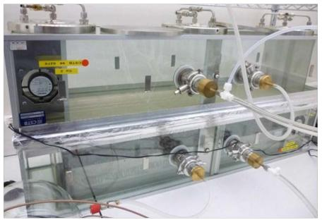
Figure 11: "Attic scenario" experimental test chamber (CSTB 2013)
