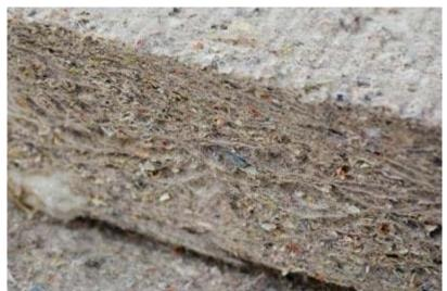
Figure 6: Illustration of cellulose insulation panels
