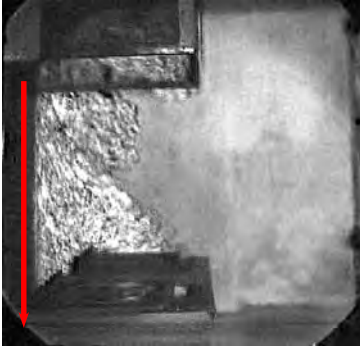
Figure 8. Schlieren image shows the thermal plume being pulled captured with backwall supply.
