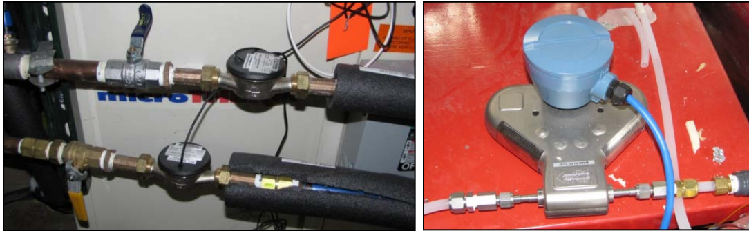
Figure 6. Inlet turbine flow meters (left) and coriolis flow meter for condensate (right).
