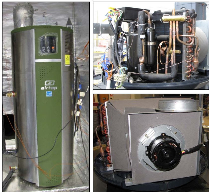
Figure 32. Unit E installed in test plenum (left). Some of the refrigerant system is shown (upper right), along with the blower that is designed to connect to a 6" duct (lower right).
