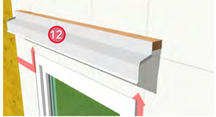
12. Install head flashing using wood blocks to space it beyond the insulation layer.
