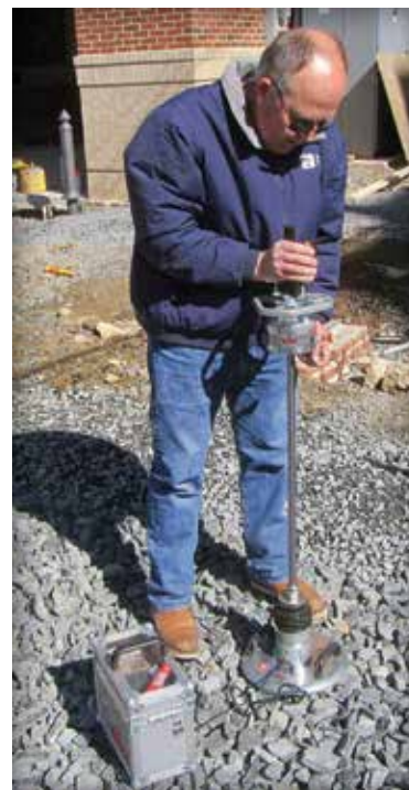
Figure 22. Testing base stiffness using light-weight deflectometer.
