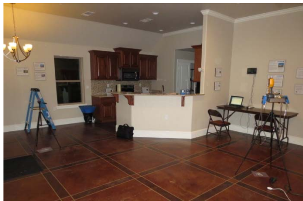
Figure 14. House 2 Main zone with PFT source tripod on left and sampling station tripod on right
