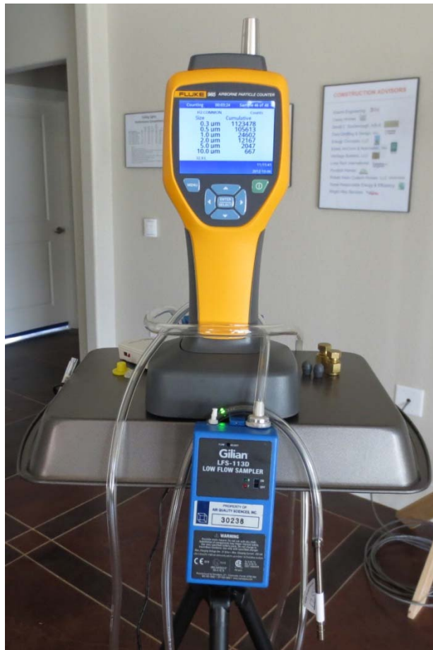
Figure 18. VOC sampling pump and solid sorbent sample tube; airborne particulate counter on top of sampling fixture
