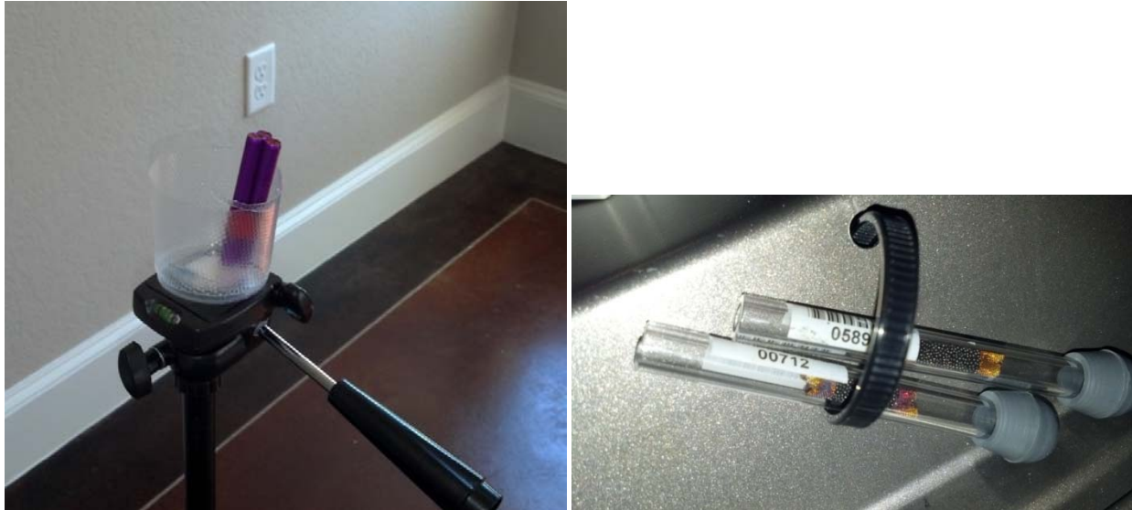
Figure 15. PFT source (left) and primary and backup CATS (right)
