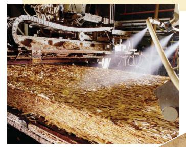
**Strength in numbers.** Each layer of thin, narrow wax-and-resin-coated wood strands is arranged with its grain direction oriented 90° to the layer below, just like plywood. The cross-lamination of thousands of strands provides strength in both directions without knots or voids in the panel. Spray nozzles maintain proper moisture content until the mat reaches the press.
