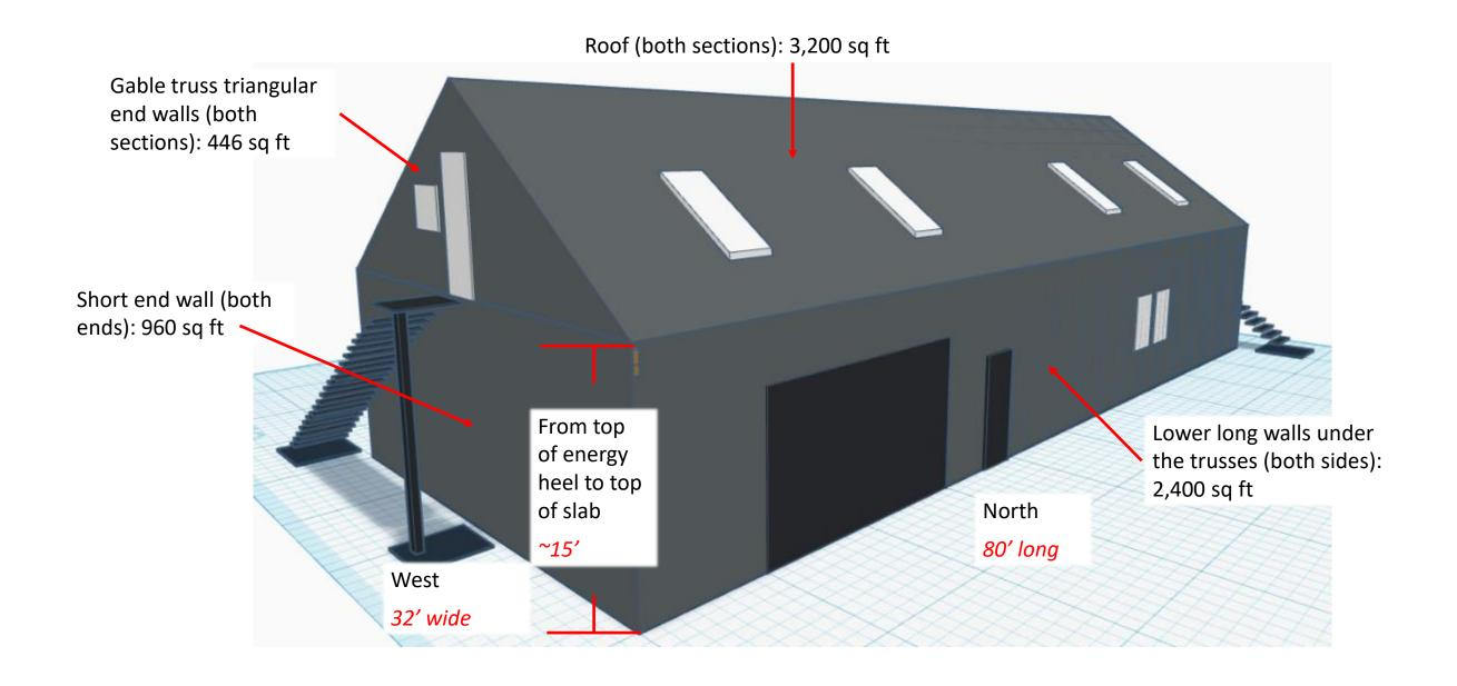
Very rough concept rendering. Placements of fenestrations are not to scale. Placement of wall studs are not to scale. Skylights will be Velux roof windows.
