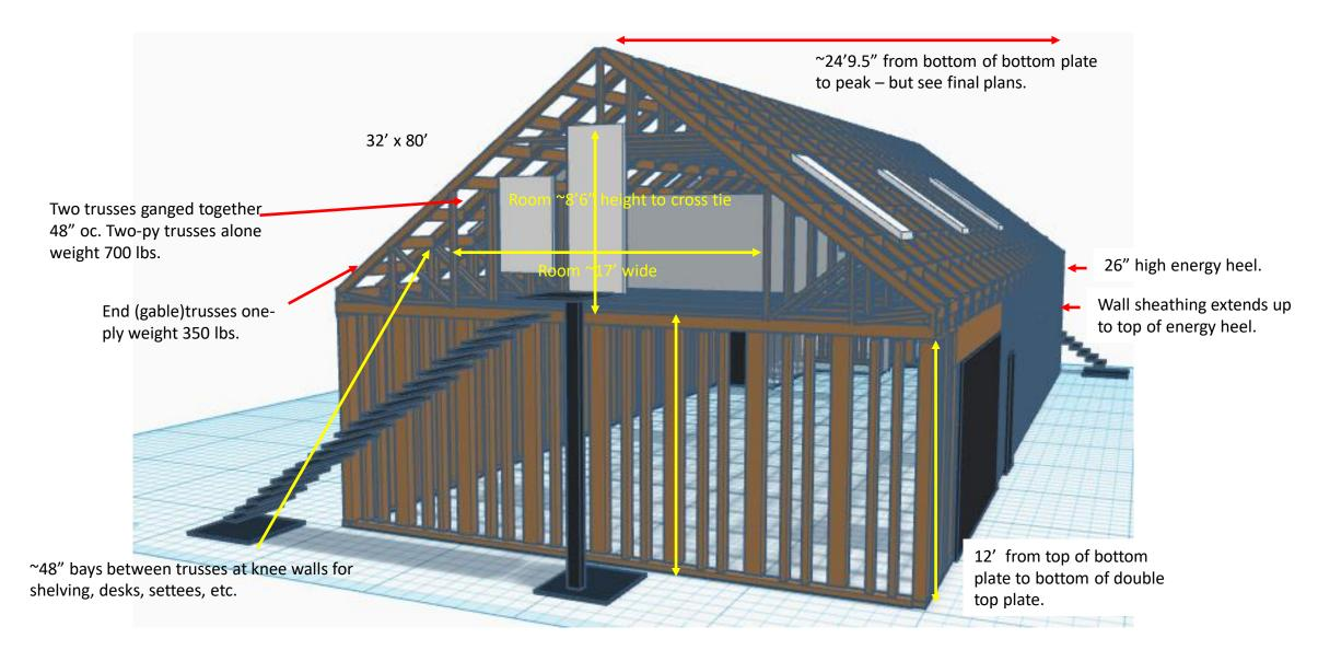
12' 4.5" from slab to top of double plate.
