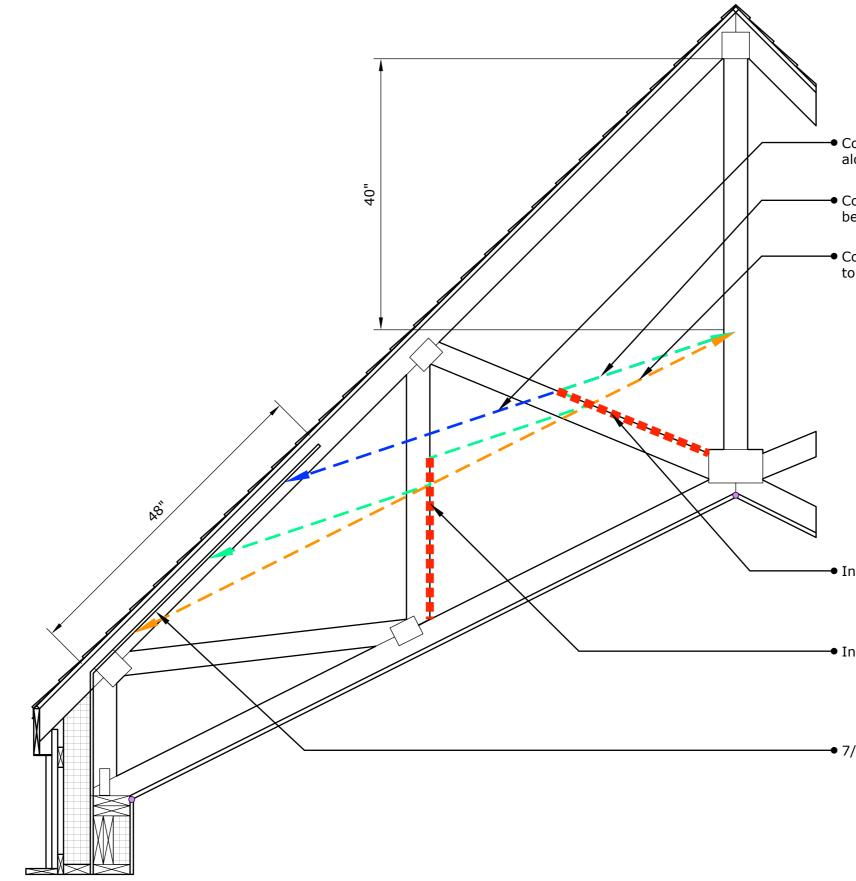
Condition A: 18" blown in cellulose, slumped along 4:12 pitch
