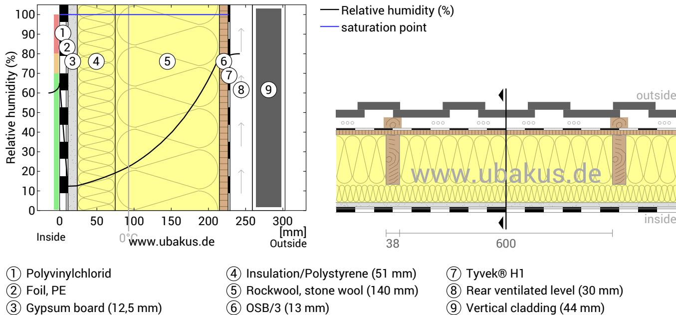
Notes: Calculation using the Ubakus 2D-FE method. Convection and the capillarity of the building materials were not considered. The drying time may take longer under unfavorable conditions (shading, damp / cool summers) than calculated here.
