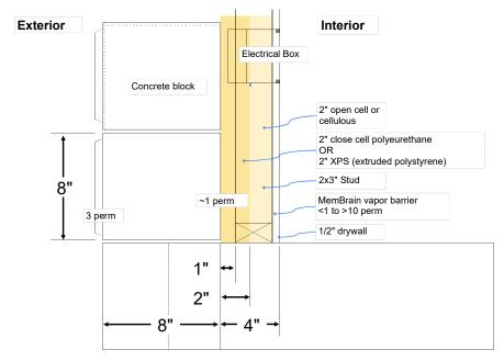
Concept 03: Closed Cell Foam (SPF) on Concrete [R14]
