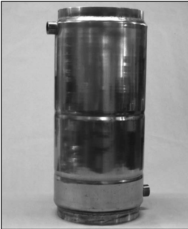
Figure 6. The Fluemiser is a section of double-wall flue pipe that works as an air-to-water heat exchanger. Water circulating through the stainless-steel cylinder is heated by warm flue gases.
