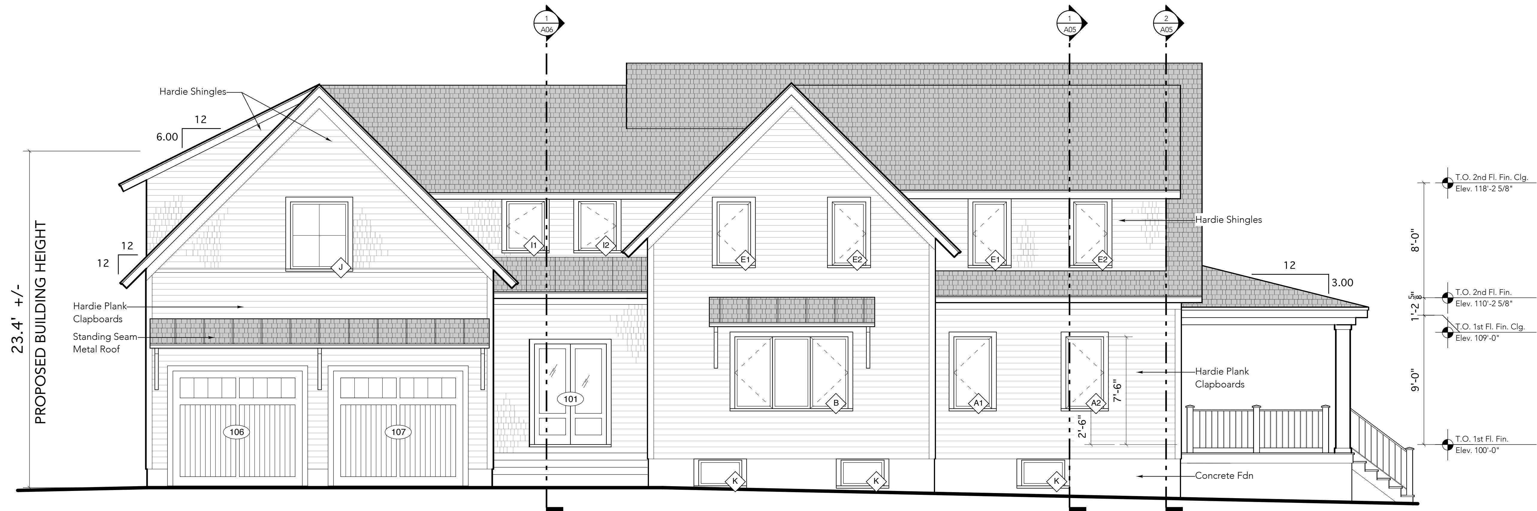
1 Front Exterior Elevation - NORTH SCALE: 1/4" = 1'-0"
